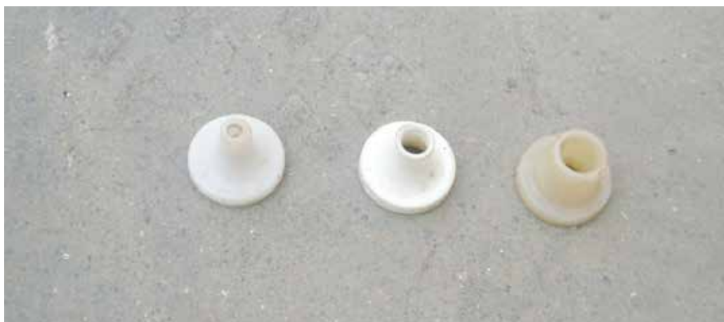
Picture 12. High, medium and low pressure jets
