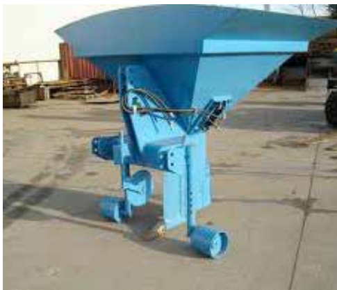
Picture 26. Gravel Mole plough showing hopper
