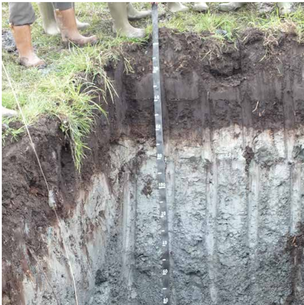
Picture 23. Test pit excavation
