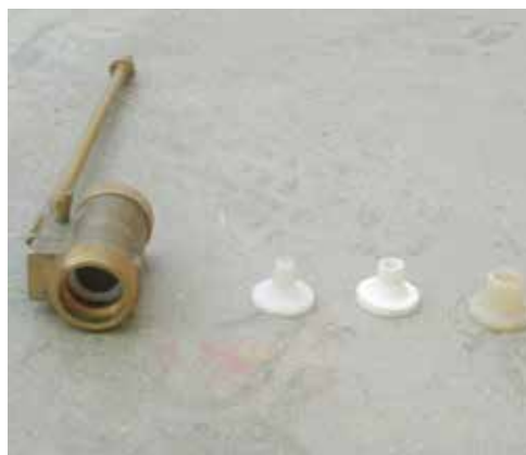
Picture 14. This is a bulkier version of the 1/2 inch ballcock, in which fits the low pressure jet as well. Note the bigger seating gasket for the jet inside
