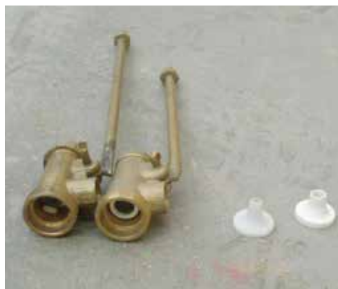
Picture 13. Two standard 1/2 inch ballcocks, one showing a shorter float arm. High and medium pressure jets can be used with this type of ballcock
