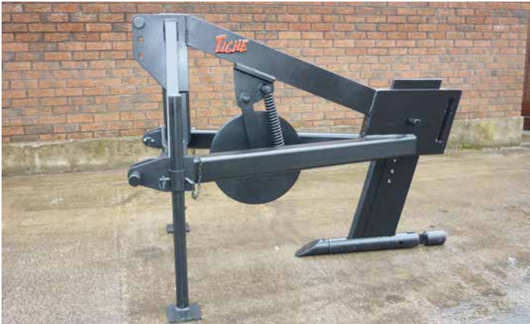
Picture 25. Mole plough showing cylindrical foot and expander
