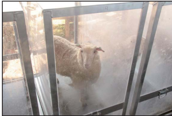
Figure 1. Portable accumulation chambers for the measuring methane in sheep
