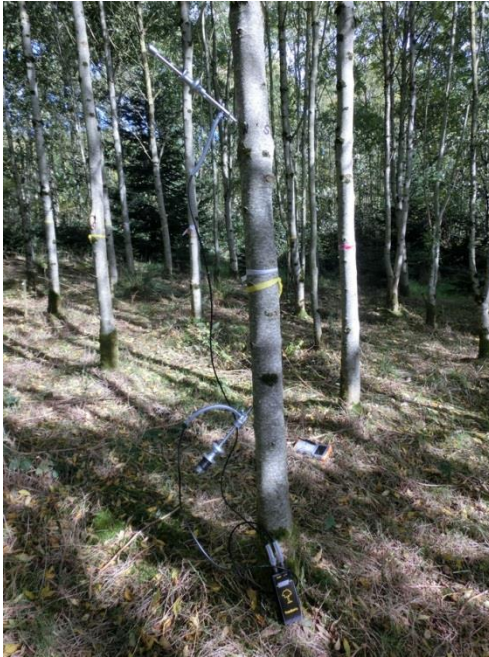
Figure 1. Non-destructive testing of standing ash thinnings using TreeSonic equipment.
