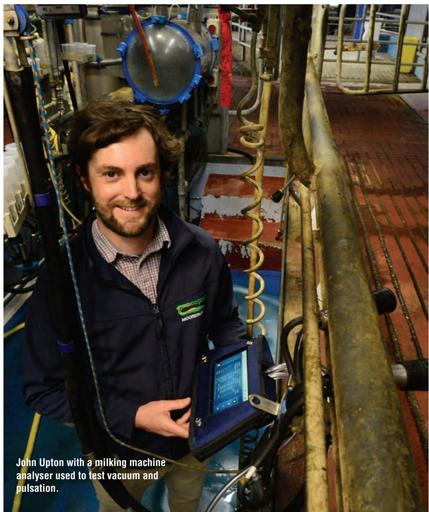
John Upton with a milking machine analyser used to test vacuum and pulsation.
