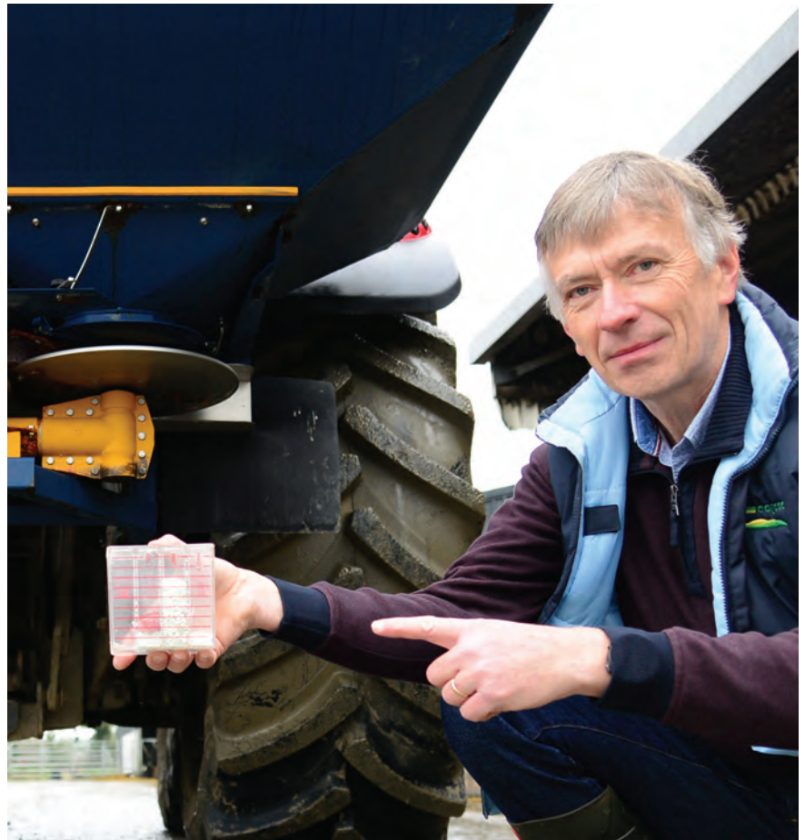
Modern spreaders enable the spreading elements to be set to suit fertiliser physical quality and the bout width. Headland spreading mechanisms also need to be adjusted.
