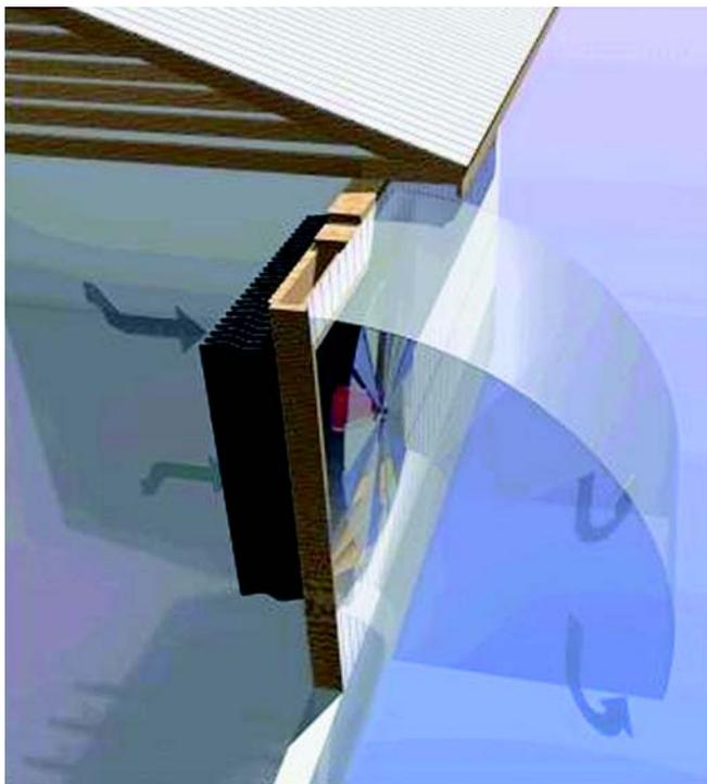
Figure 3. Light-blocking fan cover.
