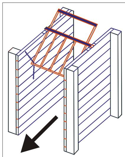
Figure 10-12: One type of a one-way gate (BORG, 1994).
