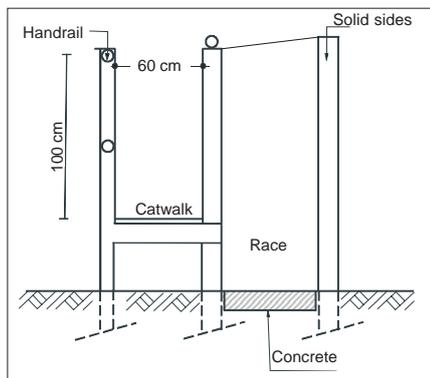
Figure 10-9: Cross-section of a catwalk with handrails.
