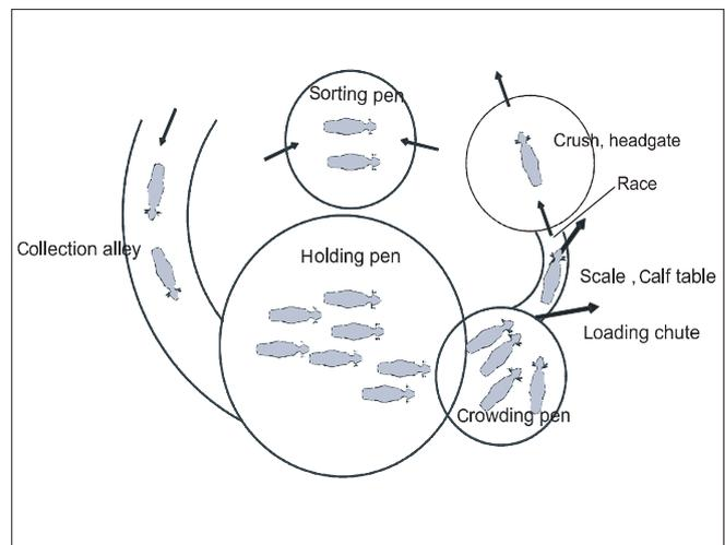
Figure 10-2: Components of a cattle-handling system (BORG, 1994).
