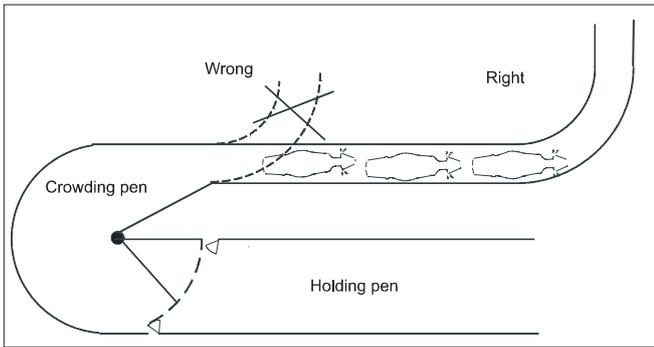
Figure 10-3: Layout for a curved handling system. If the single file race is bent too sharply where it joins the crowding pen, the cattle may refuse to enter, because it looks like a dead end. Cattle standing in the round crowding pen must be able to see a minimum of three body lengths up to the single file chute before the curve begins (GRANDIN, 1999<sup>b</sup>)
