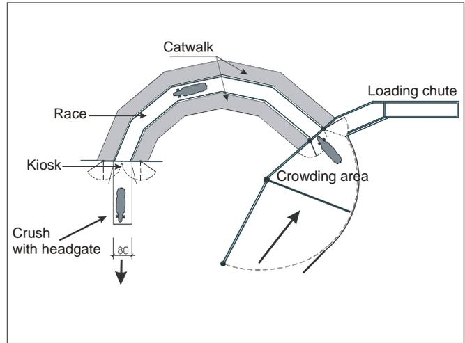
Figure 10-4: Basic Layout for a working unit
